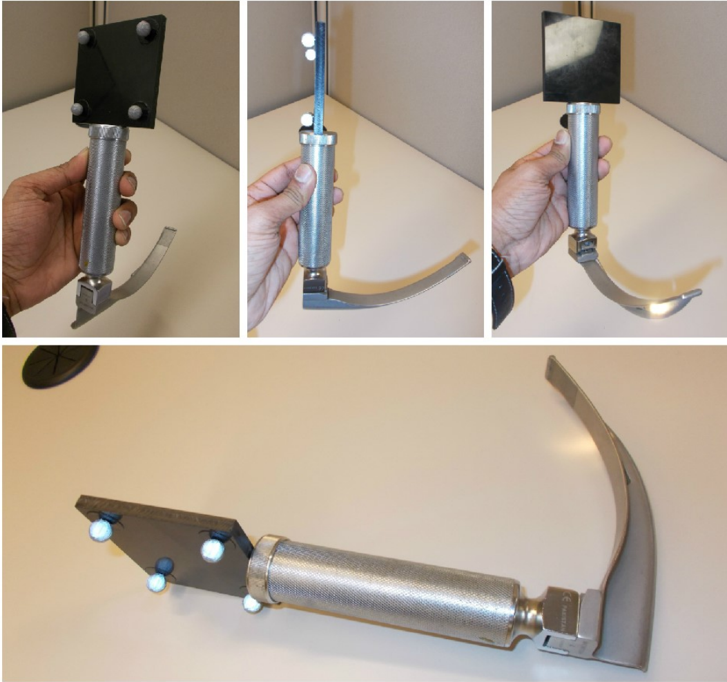
Figure A.5. Modified Laryngoscope with Reflective Markers
